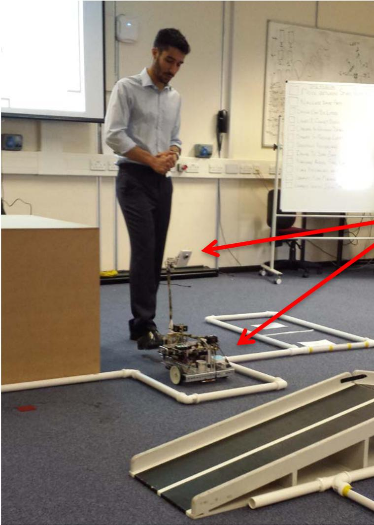
Robot with wireless camera with a TP-Link Nano router to send video streams from robot to remote computer.
