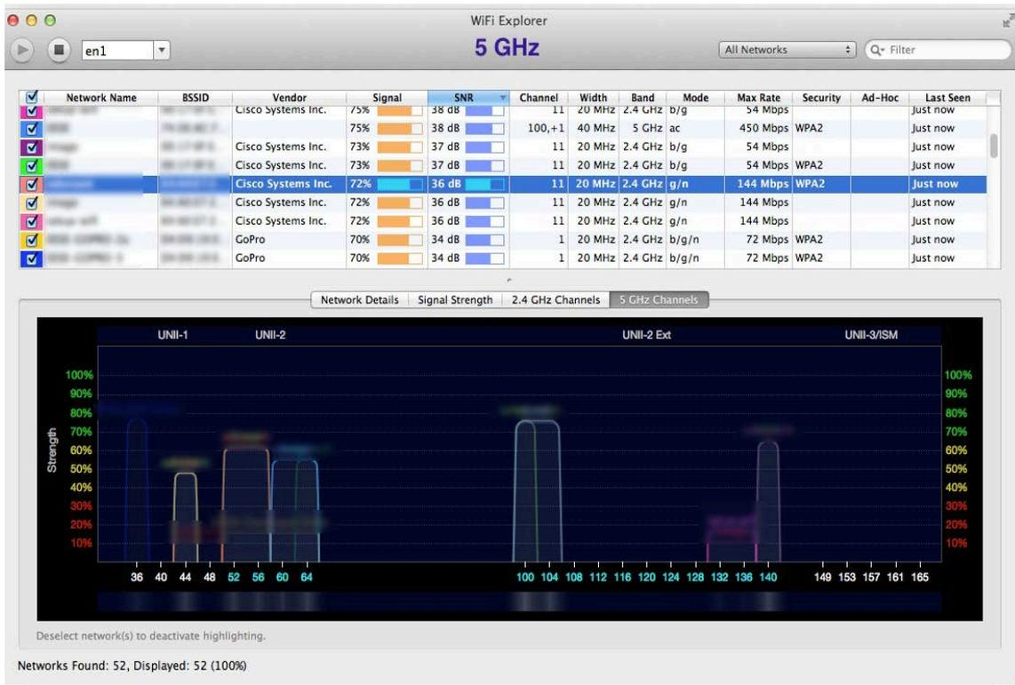
To provide more of a resilient workable solution, improving robustness of the service to help minimise impact of any future interference and eliminating the number of frequent dropouts, it was decided that all future demonstrations should use 5GHz with supported 802.11ac support.
